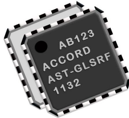
AST-GLSRF follows a typical super-heterodyne architecture. It has an on-chip LNA as the first block with a typical gain of 20dB and Noise figure of 2dB. This is followed by a single mixer stage which down-converts the input signal frequency band of GLONASS satellites to a manageable IF frequency of 2.46 to 9.77MHz. The IF amplifier and low pass filter stages that follow ensure that the IF signal is suitably amplified and filter the unwanted out of band interference.
