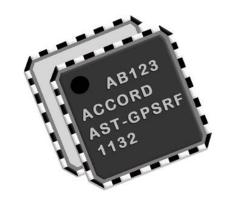
AST-GPSRF is a high performance, fully integrated GPS / Galileo RF front-end chip for down conversion and signal amplification. It is designed for GPS L1 (1575.42MHz), C/A and Galileo OS (1575.42MHz) receivers. It can also process the signals from SBAS satellites.
