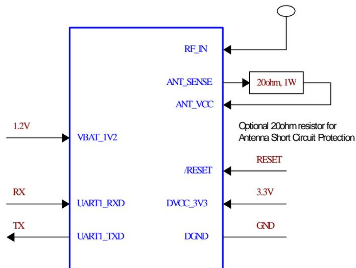
Figure 2: Circuit Interconnection using Navika-150 module
