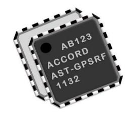
AST-GPSRF is a high performance, fully integrated GPS / Galileo RF front-end chip for down conversion and signal amplification. It is designed for GPS L1 (1575.42MHz), C/A and Galileo OS (1575.42MHz) receivers. It can also process the signals from SBAS satellites.
