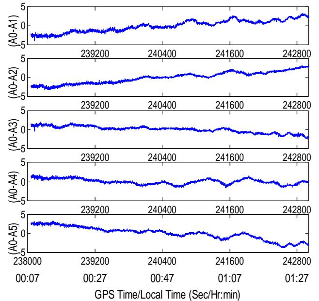
Figure 11: Single differenced residual carrier phase error before applying multipath correction for SV 31 on August 25 (Y-axis in cm; A0-A $n$  denotes single difference between antennas 0 and  $n$ ).
