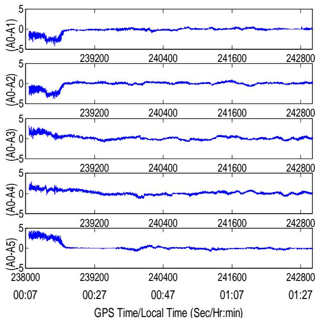
Figure 12: Single differenced residual carrier phase error after removing carrier phase multipath for SV 31 on August 25 (Y-axis in cm; ; A0- $A_n$  denotes single difference between antennas 0 and  $n$ ).
