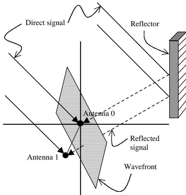
Figure 1: Correlated multipath errors can be related to each other through signal direction and known geometry between the antennas.
