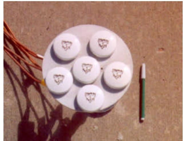
Figure 3: Antenna array assembly.
