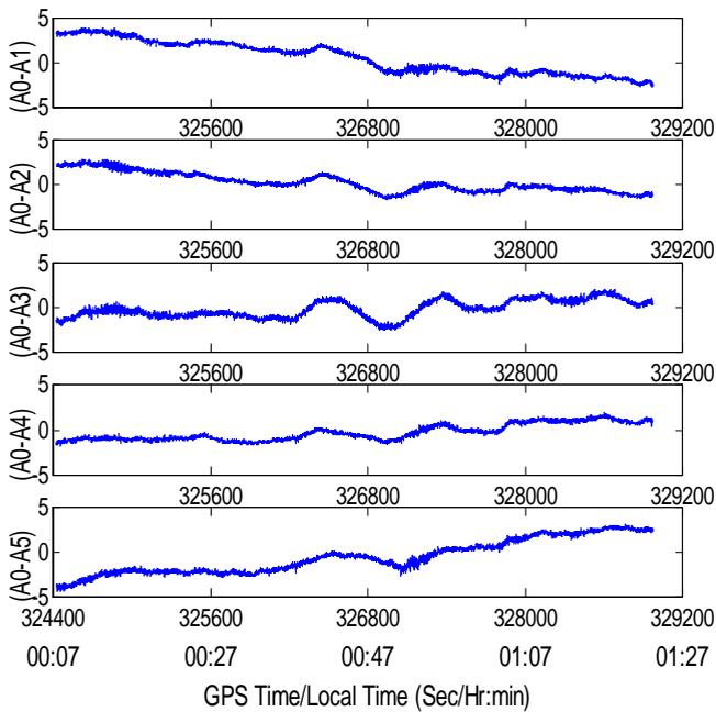
Figure 6: Single difference residual carrier phase error before applying multipath correction for SV 21 on August 26 for the same time of day (shifted by 4 minutes) as in Figure 5 (Y-axis in cm; A0- $A_n$  denotes single difference between antennas 0 and  $n$ ).
