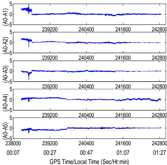
Figure 9: Single difference residual carrier phase error after removing estimated carrier phase multipath for SV 21 on August 25 (Y-axis in cm; A0-A $n$  denotes single difference between antennas 0 and  $n$ ).
