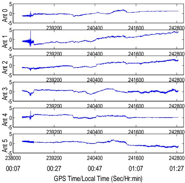
Figure 8: Estimated carrier phase multipath error for SV 21 on August 25 for each antenna (Y-axis in cm).
