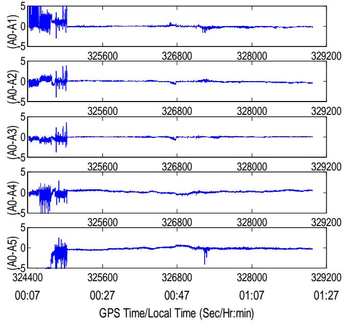
Figure 10: Single difference residual carrier phase error after removing estimated carrier phase multipath for SV 21 on August 26 (Y-axis in cm; A0-A $n$  denotes single difference between antennas 0 and  $n$ ).
