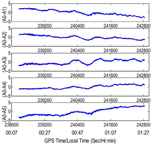
Figure 5: Single difference residual carrier phase error before applying multipath correction for SV 21 on August 25, 1998 (Y-axis units in cm; A0- $A_n$  denotes single difference between antennas 0 and  $n$ ).
