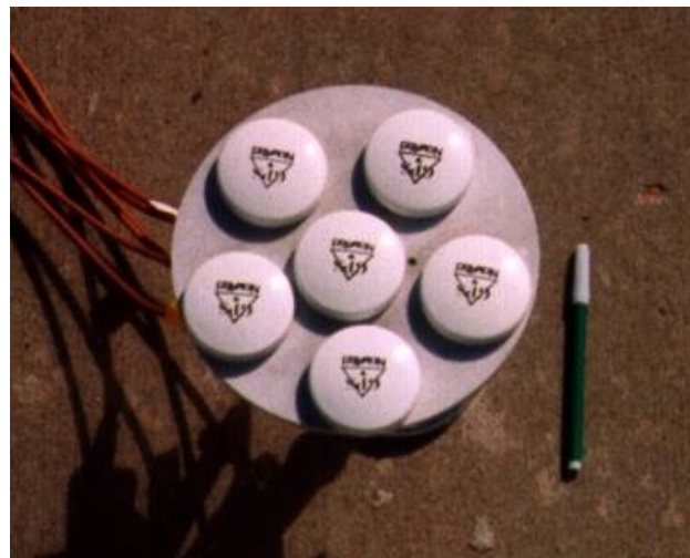
Figure 4: Antenna array assembly.
